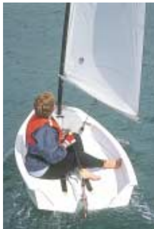
The false floor allows greater cockpit space.
