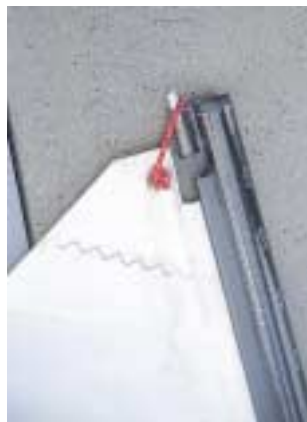
Halyard lock is a simple spring-loaded pin.
